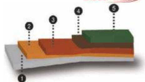
5. **POLYSPORT XP 1069 - UV-resistant, two-component, universal, mat, top coating for the protection of EPDM granules.**
